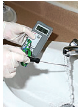
Temperature Check of Water Should be 50°C after 1 Min
